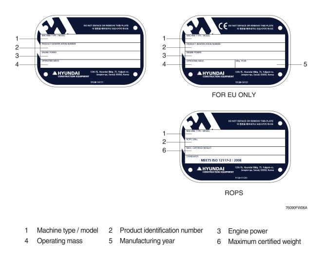
\* The product identification number assigned to this particular machine and should be used when requesting information or ordering service parts for this machine from your authorized HYUNDAI dealer. The product identification number is also stamped on the frame.
